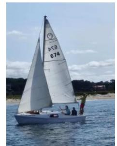
The Islander (a masthead, sloop rigged, monohull) is an early fiberglass constructed boat designed and built by Joseph McGlasson from 1965 to 1969. McGlasson built popular wooden boats in the mid-1950s and it is said that the planking seams that can be seen on the Islander's hull is a signature feature carried over from the mold used to construct the fiberglass version of this boat. Timing: June-September 2026
